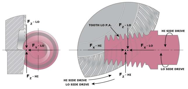
When selecting bearings, it is necessary to know the direction and magnitude of the tooth forces so that bearing relations may be determined. The tables below convey both unit- and operational-tooth loads for:
